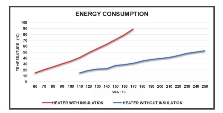
Our test has shown that the new insulated PREMIUM silicone band guarantees an average energy saving of 60% compared to other bands without thermal insulation.
